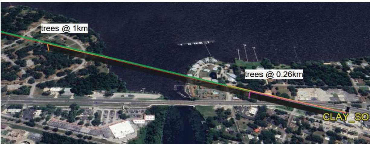
Figure 1-6: Link between the Clay County Sheriff's Office tower to the new Sleepy Hollow tower
